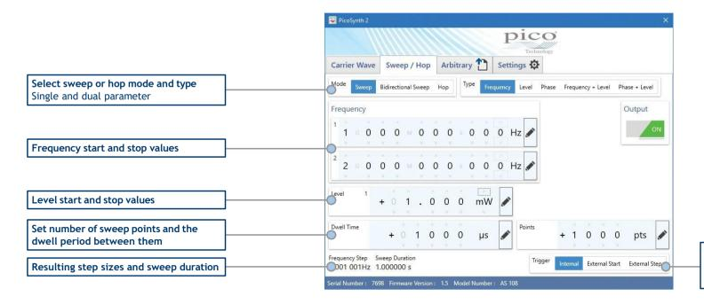
Synchronize the sweep to a trigger Internal clock, external input or software trigger sources. Trigger a sweep or trigger next point in sweep.
